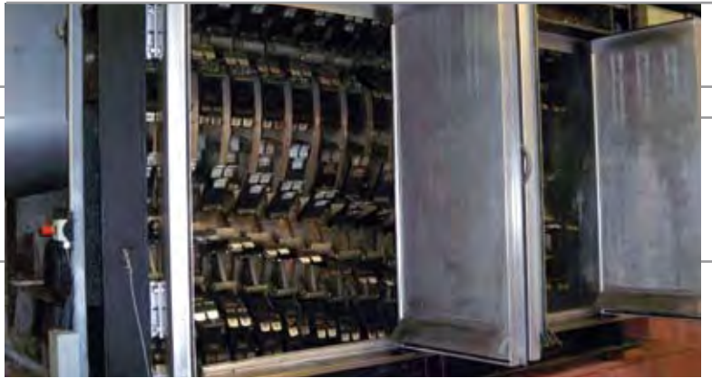
Final main de-hairer and scraper feeding out onto inspection and cutting line with bottom screw auger for waste.
