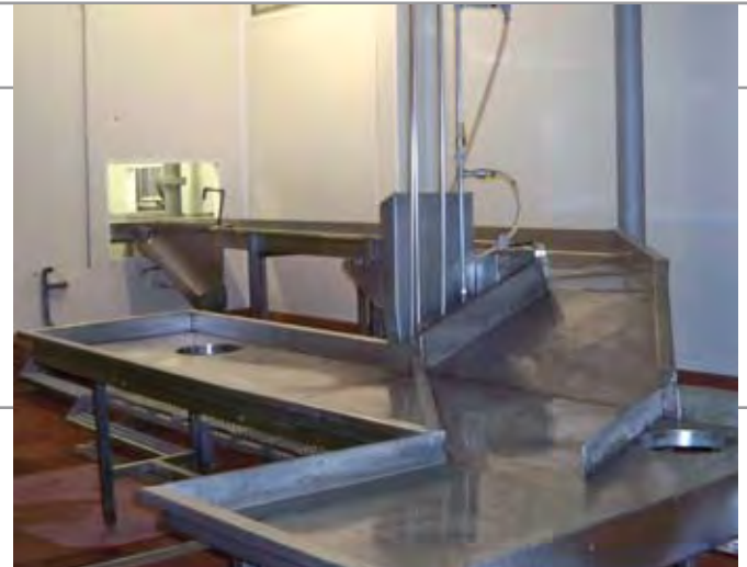
All s/s table and incline chute system for casing for natural sausages.
