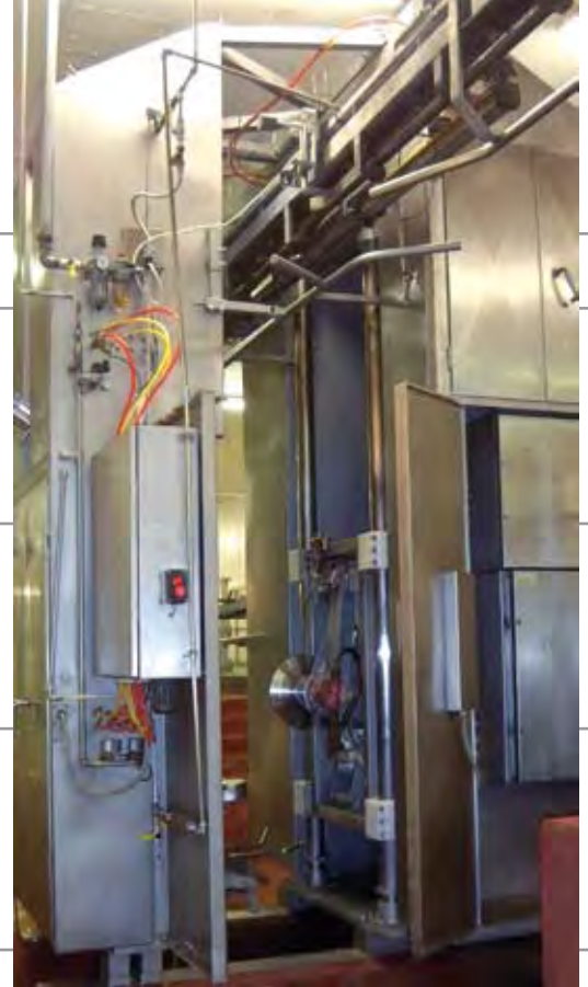
Fully automatic pig splitting system with automatic product sensors and offal removal, totally s/s.
