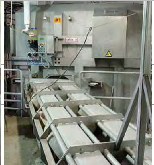
Butina Jumbo anaesthetising CO 2 auto stunner multi cradle system. Fully automatic.
