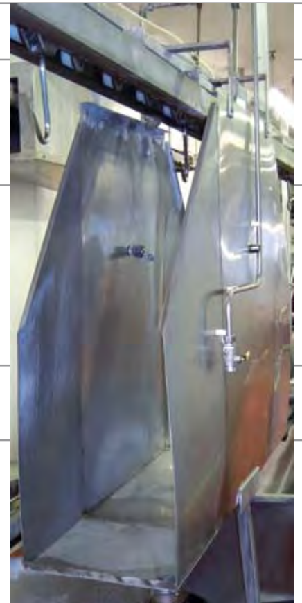
Overhead rail system and wash for offal, s/s.
