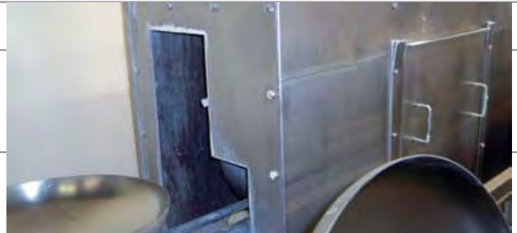
Offal tray washer system, inline, all s/s.
