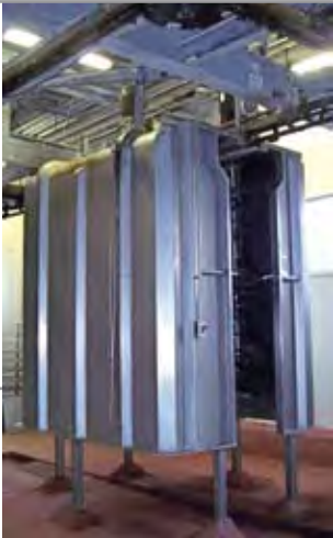
Primary all s/s flayer fed by overhead track system. Fully automatic.
