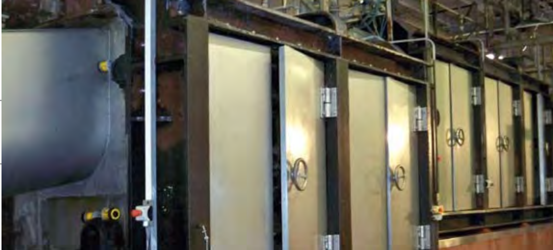
The two de-hairers leading from one to the other and end chute.
