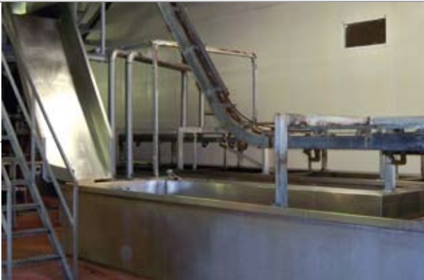
Product being fed from scalding tank and automatically unload into primary scraper and de-hairer.
