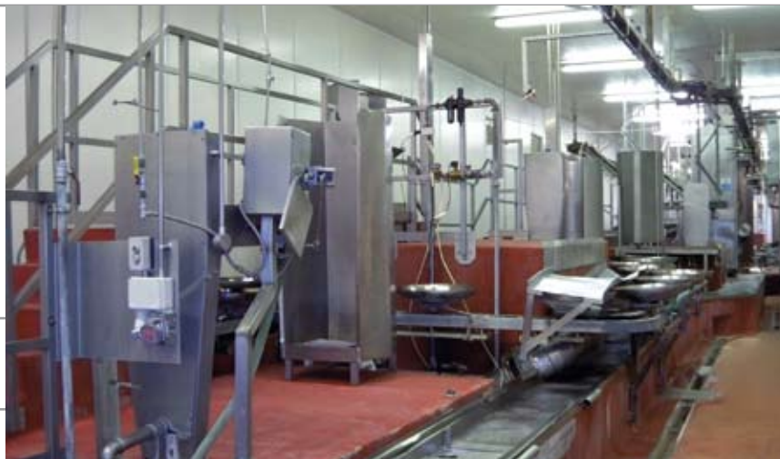
Part of the complete offal line, pig splitter and inspection work stations.
