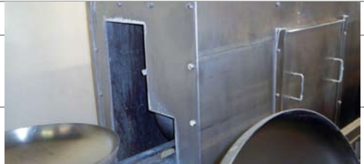
Offal tray washer system, inline, all s/s.
